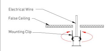
4. Raise the fixture to cutout and push the fixture in the false ceiling.
