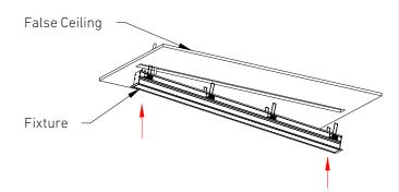
5. Use packing material if the fixture remain loose in rge false ceiling.
