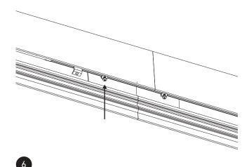
Replace the reflector using the fixing screws. Make connections between the housing and the reflectors and between each reflector section.
