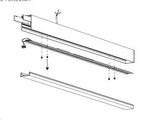
Secure the fixture to the ceiling using appropriate fixing screws. Make electrical connections.
