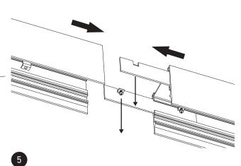
With the two fixture sections firmly pushed together tighten all the screws on the connecting plate.
